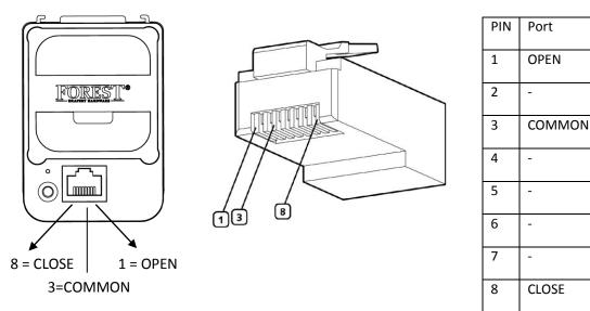
**OPEN:** Pin 1 is connected to pin 3 the motor will open the curtain
